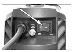
welder has cooled sufficiently (the thermal overload indicator goes out) before restarting work.
